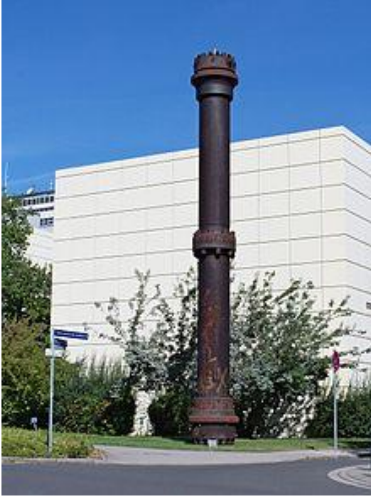
A historical (1921) high-pressure steel reactor for production of ammonia via the Bosch-Haber process on the premises of the University Karlsruhe (now KIT South Campus) Germany.
